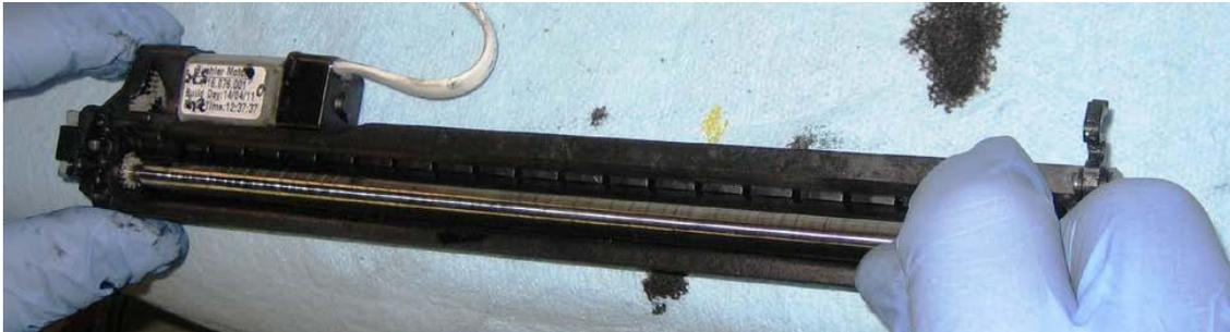
*Picture of Transfer Roller (TR)*
