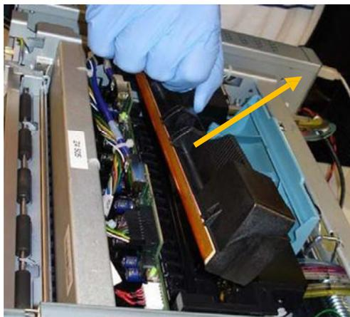
*Picture of sliding the PH out of the unit*
