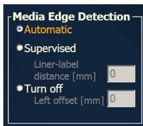
**Automatic** – by choosing this option you rely on the printer sensors to handle the material
