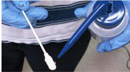
3. Place the damp swab on each sensor and twist back and forth to clean the surface. Use a new, moist swab on each sensor.
