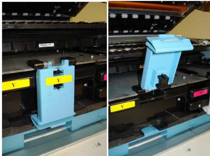
*Picture of opened and closed Int Tank Latch*
