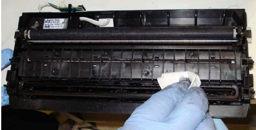
*Picture of Ink Residue removal from the Maintenance Module*
