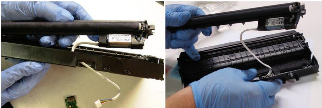
*Picture of routing ribbon cable through housing*
