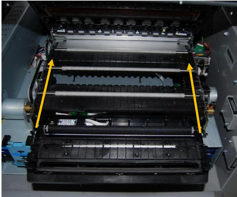
3. Slowly turn the gear on the print engine until the maintenance module engages.
