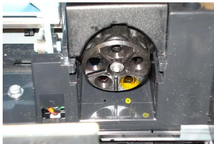
*Picture of Fluidic Coupling with ink residue*
