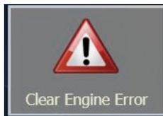
The controller attempts to discover error states and guide the user in order to recover from these. In cases when this is not sufficient or the controller failed to detect the engine error and react to it, pressing this button may help clearing engine error states (eg. after paper jam).
