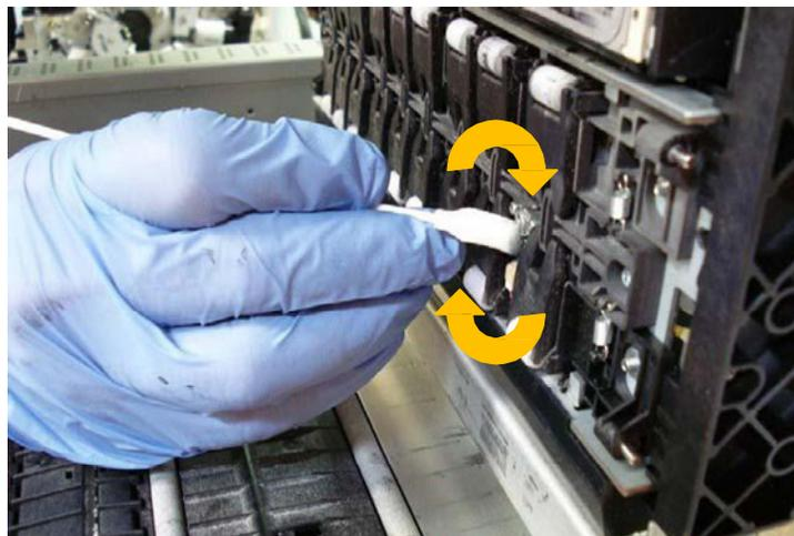
4. Repeat cleaning and drying process for all four sensors.
