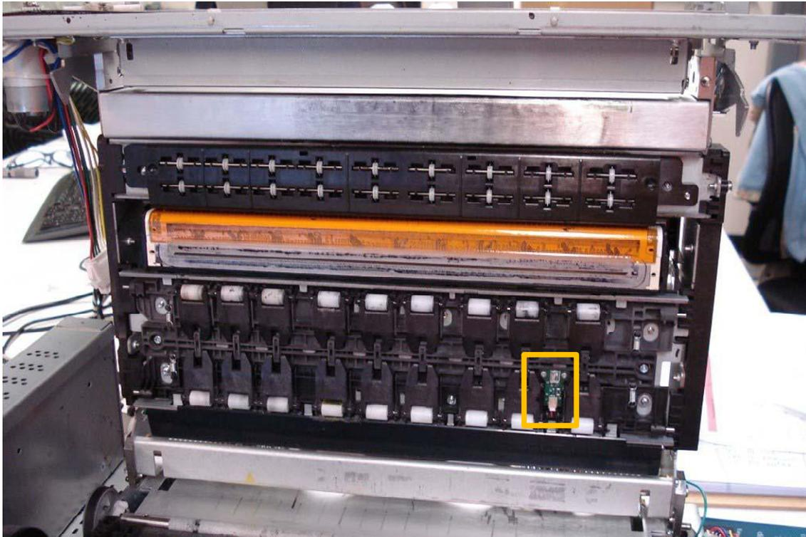
*Picture of Paper Path Optical Sensor Locations - Top*
