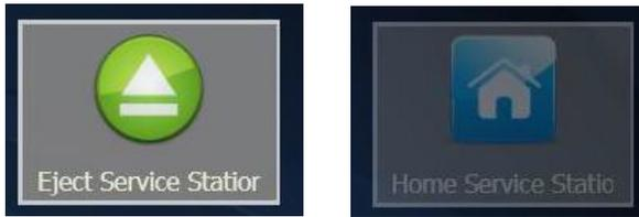
These buttons are added to provide the user/technician to eject the service station for removal and then send home the station after inspection or replacement. Home service station button will automatically replace the Eject Service station button if there is no Service Station in the printer!
