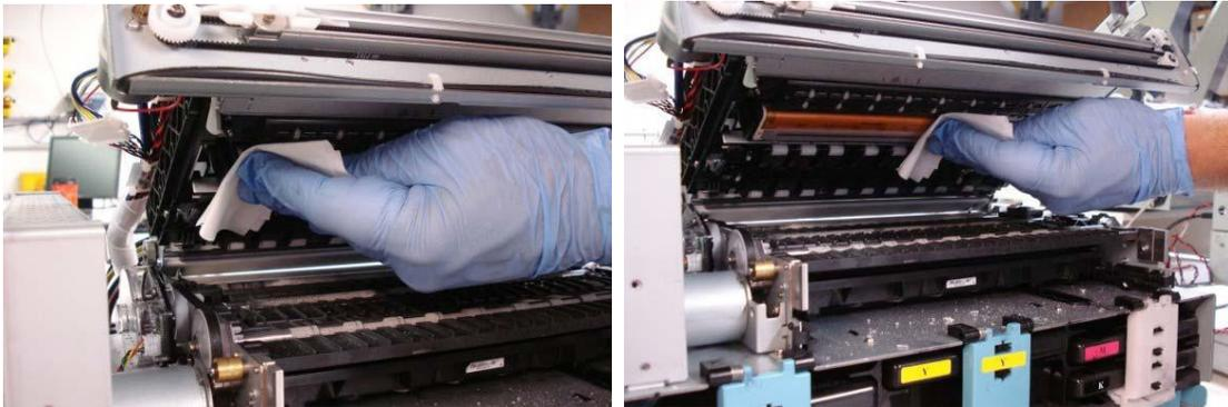
*Picture of wiping the nozzles*
