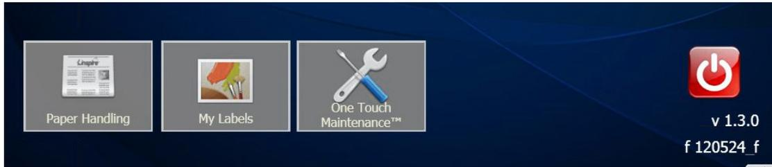
The bottom of the screen gives access to various menus. On the right, a large red virtual Power On/Off is shown. Use this button to switch off the printer! Under this button the two values are the version of Liberty and the version of the firmware.
