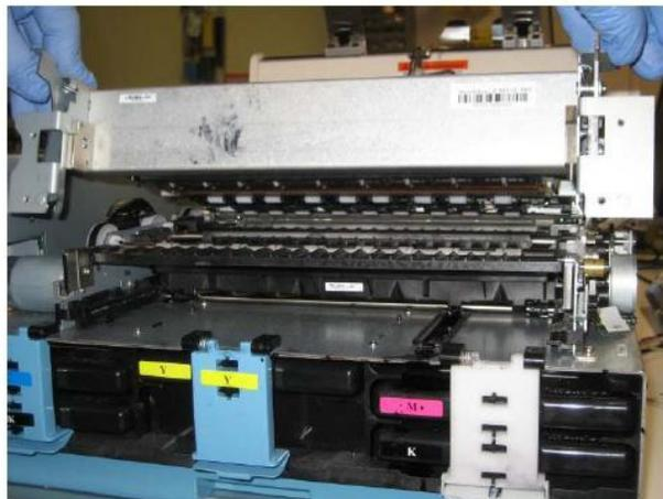
**NOTE:** The wiper is automatically in the up position when the clamshell is open.
