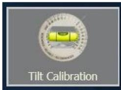
The printer has built-in tilt sensor which should be calibrated once the printer is properly installed. It should also be recalibrated if the unit is moved.
