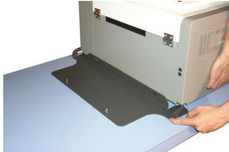
basement to the printer and fix with the two knobs.
