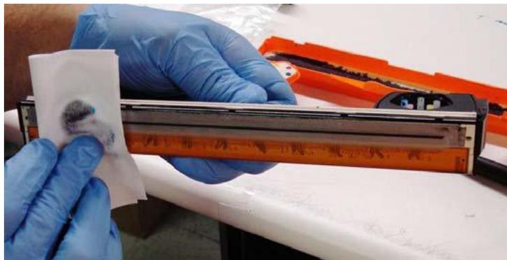
*Picture of wiping PH nozzle strip*
