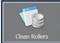
This button will move the paper back and forth in the print zone in an attempt to clean the rollers, thus preventing contamination of the printed labels afterwards.
