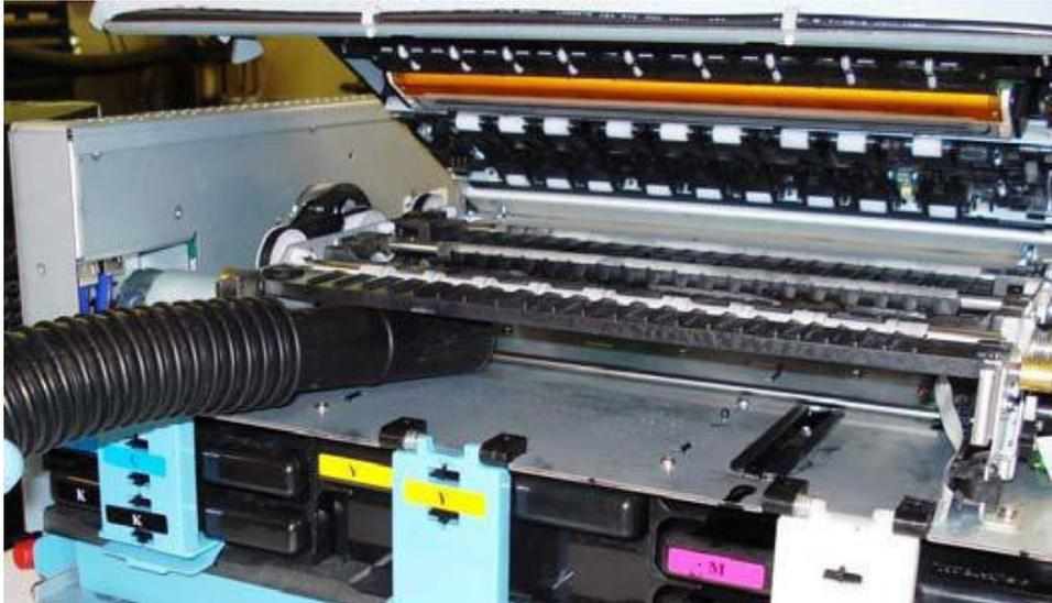
*Picture of using a Vacuum cleaner to remove debris from under the MM*
