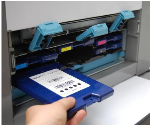
*Picture of re-installing Ink Tanks*
